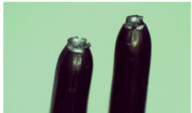
Fig. 10 Typical ductile failures for nitinol in tension—irradiated FEP-coated nitinol shown
